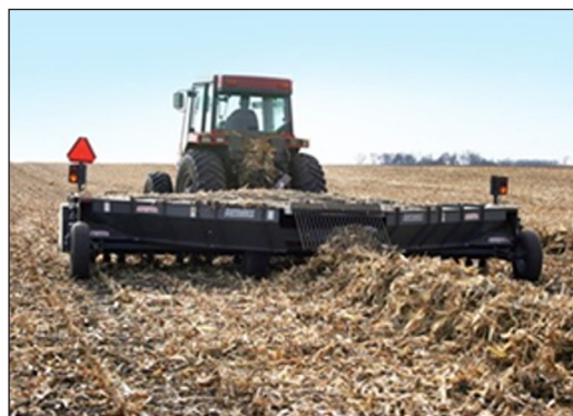
This modern center-discharge shredder is pretty much a dead ringer for the machine that Kent and I cobbled together in the early 80s for windrowing corn stalks. (Loftness Manufacturing)
